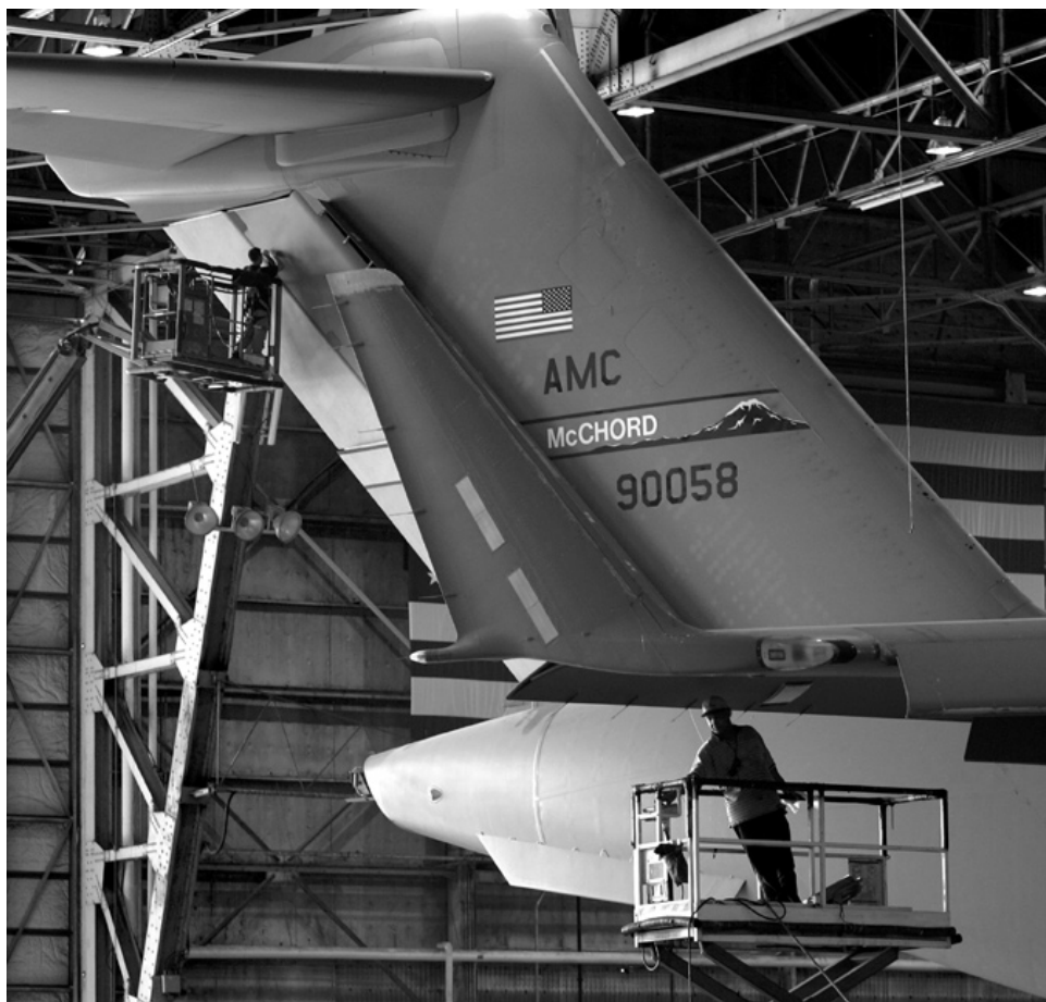
Employees use lifts to get to upper sections of military aircraft being maintained at Boeing's San Antonio facility at KellyUSA.
