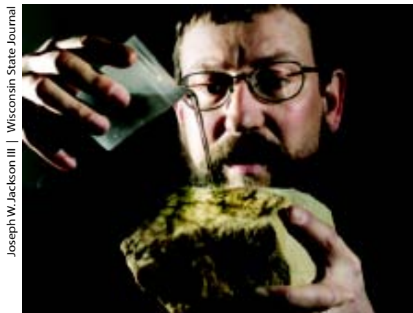
In addition to investigating contaminants in drinking water, stories explained how the local water system works. Here, hydrologist David Hart demonstrates how a piece of the Mount Simon sandstone aquifer soaks up and stores water.
