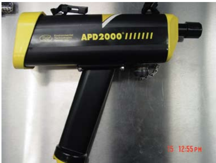
Ion mobility spectrometers can detect nerve and blister agents used in a possible chemical attack, including mustard gas. This one was purchased by the city of Burbank with federal homeland security grants.
