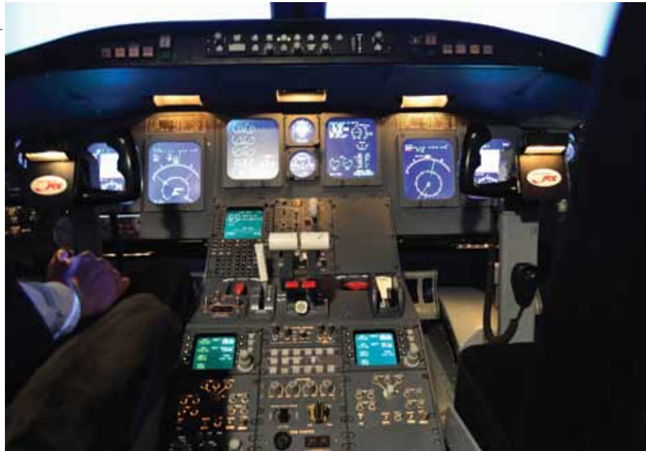
A simulated Canadair Regional Jet flight deck at Embry-Riddle Aeronautical University in Daytona Beach, Fla. The CRJ-200’s mode control panel is used to set automated flight control systems.
