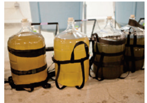
Researchers gathered runoff from a highway in Seattle to study the impacts of and possible solutions to stormwater runoff. The darker colored carboys contain straight highway runoff. The lighter ones contain runoff filtered through soil columns.
