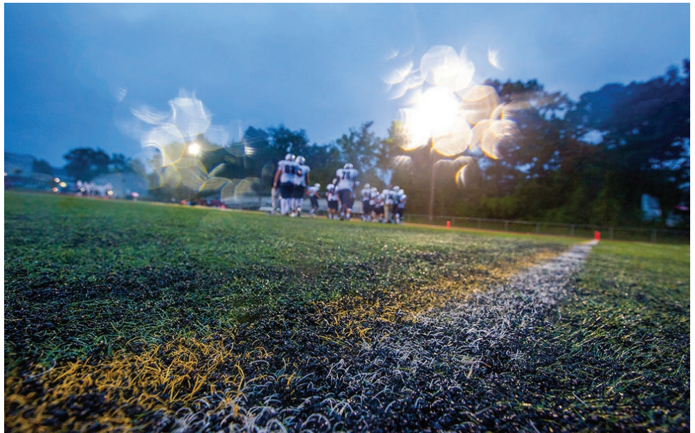
Once lush and standing up, fibers on many Duraspine fields now look like these at Highland Park High School in New Jersey. In some areas, fibers have sheared off.
