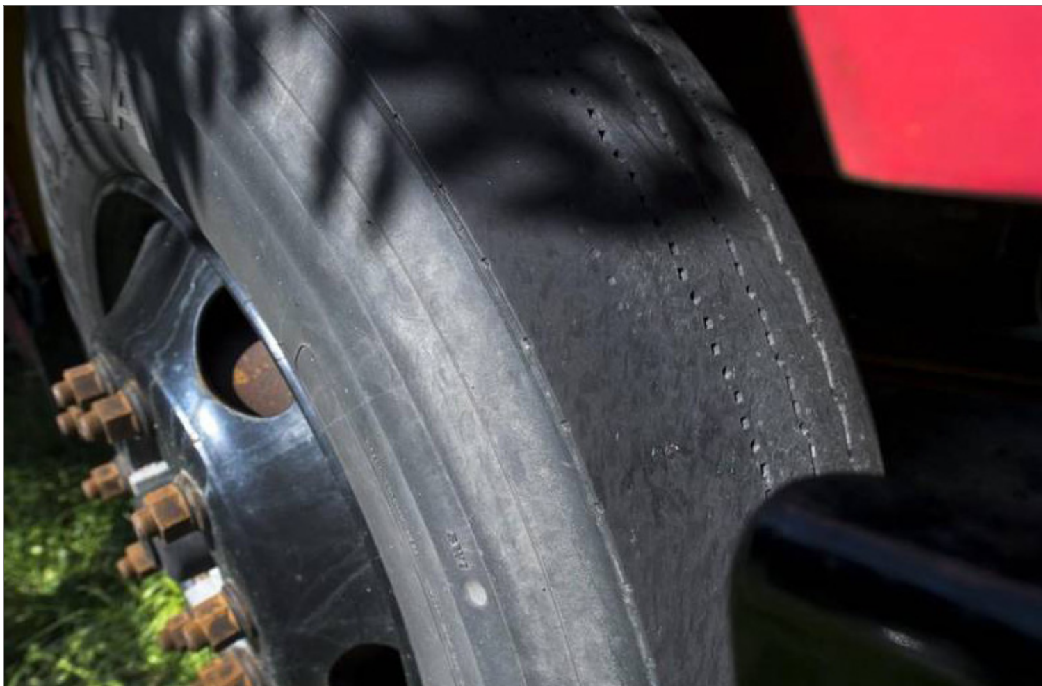
Reporters found several problems with Bus 58, including a bald front tire. Inspectors say worn tires are a critical safety issue that could have catastrophic consequences. (Keith Myers/The Kansas City Star)
